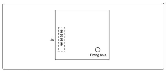
Figure 4.5 Pin layout of connector J6
